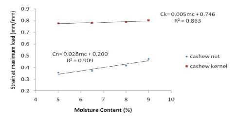
Figure 12. Variation in compressive strain of cashew nut/kernel with moisture content
