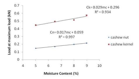
Figure 9. Relationship between maximum load of cashew nut and kernel and moisture content
