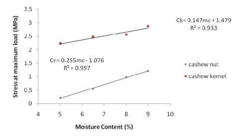
Figure 11. Variation in compressive stress of cashew nut and kernel with moisture content
